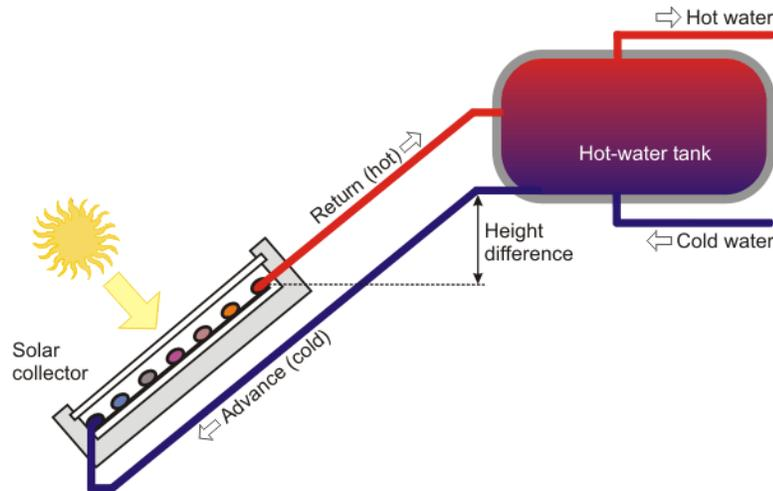
*\*This image, published in Renewable Energy World, shows how a thermosyphon passive solar water heater works*
