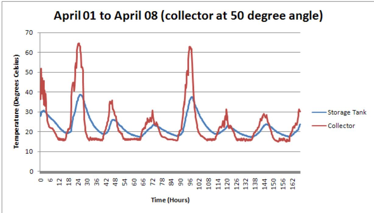
This chart represents the third week of our experiment. We chose to position our solar collector at 50 degrees this time to see if we could observe a difference in efficiency with a slightly sharper angle.
