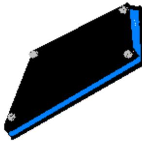
Drill four holes in each of the aluminum sheets on the corners the same size as the bolts and nuts. Place the connected tubes on the painted side of one aluminum sheet and place the other aluminum sheet on top of the tubes with the painted side facing up. Bolt the sheets together making sure to have the nut on the top and the bolt on the bottom so you are able to unscrew the nut incase a problem occurs once it is place inside the box.
