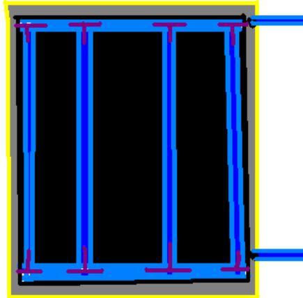
To put your bolted aluminum tubes inside the box, make sure the nuts are on the top, and start with the 30 inch size tubes and pull them through the holes you have made in your box on the right side. Then, once you have pulled the tubes completely through the foam padding and the cardboard box, push down on the aluminum, making sure it is flat on the bottom of the box, and fitted tightly inside. Place the Plexiglas on top of the box, and tape it so that it will stay in place.
