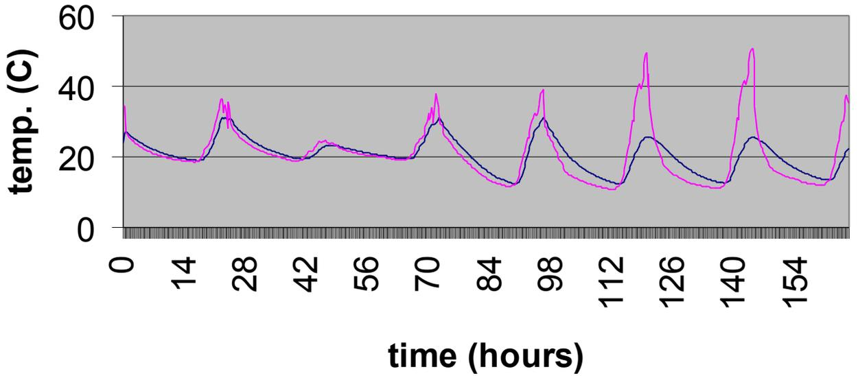
— water temp in tank — air temp. in collector
