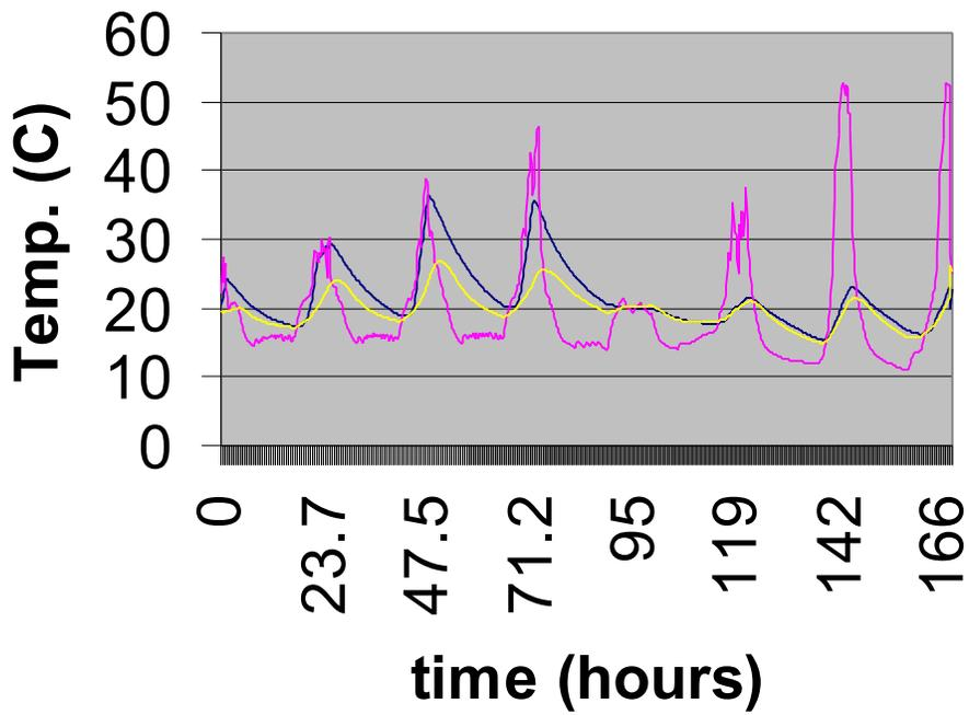
— Water temp in tank — collector air temp — air temp underneath the tank
